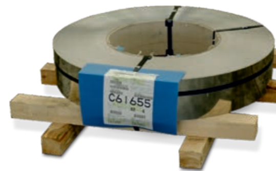
Example of packaging for eye-to-the-sky coils (V1)
